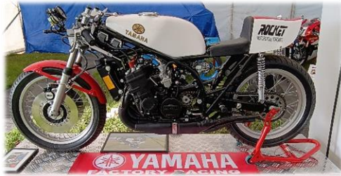
1975 was the first year at 750cc and the last year of the twin shock chassis
